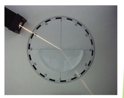
Light changes direction when encountering another transparent material with different index of refraction
