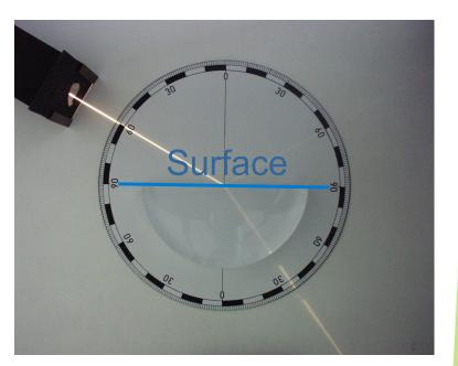
Light changes direction when encountering another transparent material with different index of refraction
